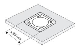
Warning! Once the metal screening has been removed, the sensor can no longer be embeddable mounted.
